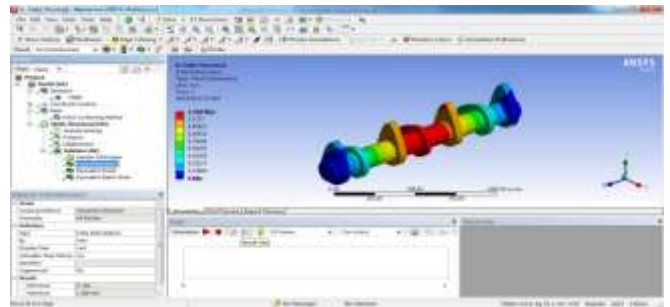
Figure 5.4: Static structural total deformation of forged steel
